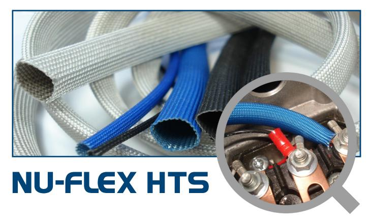
NU-FLEX HTS is a fiberglass braided sleeve that has been heat treated to remove all organic contaminants and then saturated with an acrylic binder.
